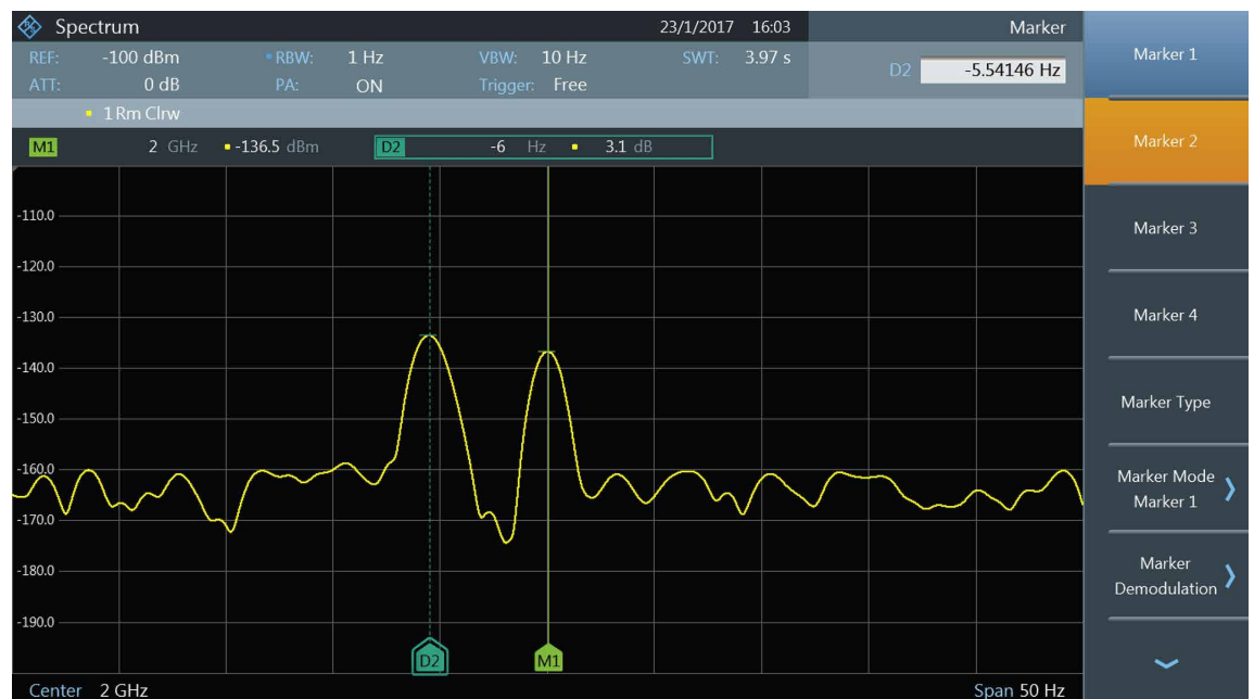
Fig. 1: The R&S®FPC1000 sensitivity with the optional preamplifier is typ. -165 dBm at a resolution bandwidth of 1 Hz.
