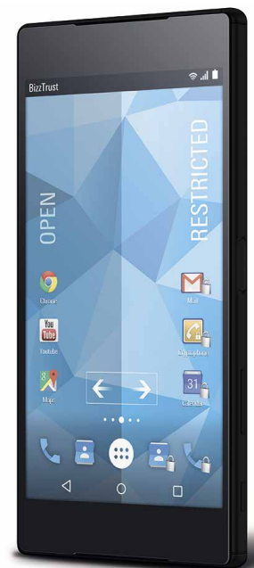
Fig. 1: BizTrust is based on commercially available Sony Android devices. A special app on smartphones also allows encrypted phone calls.
