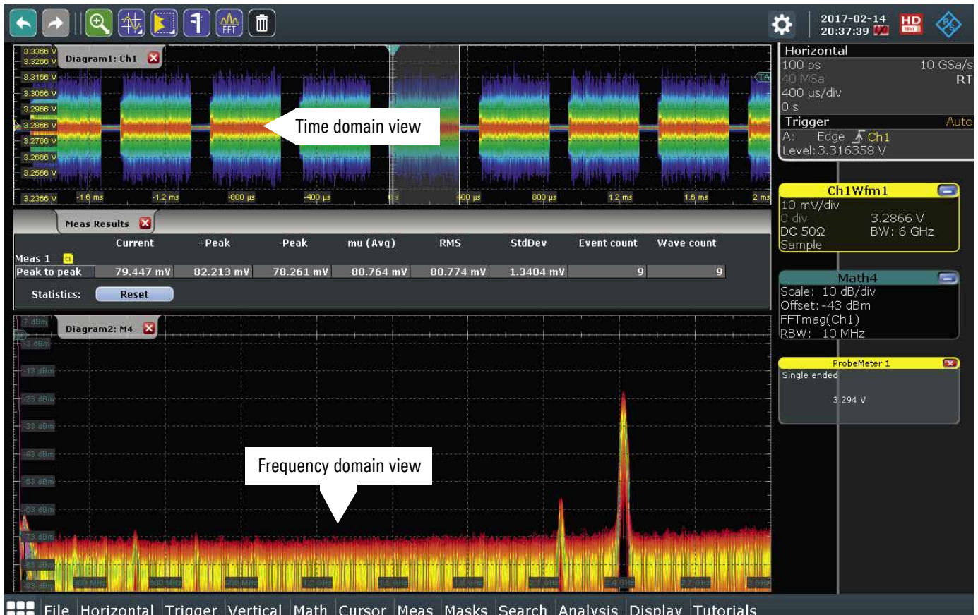
Fig. 6: The spectrum analysis function in Rohde&Schwarz oscilloscopes is a powerful tool for identifying unwanted coupled signals in DC power distribution networks. In the example, a coupled 2.4 GHz WLAN signal is clearly visible.
