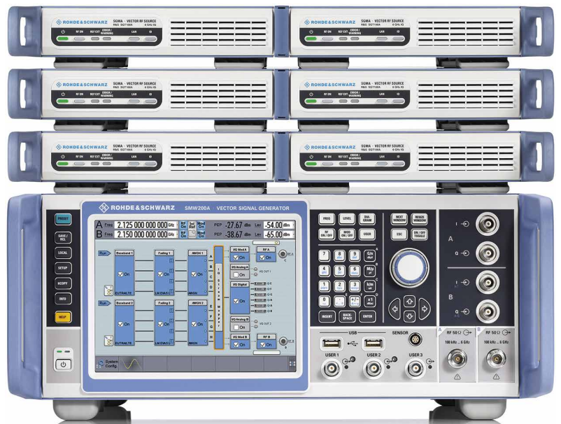
Fig. 13: Compact MIMO system for creating eight TX or eight RX signals using an R&S®SMW200A vector signal generator and six R&S®SGT100A extension units, optionally with real-time fading simulation.
