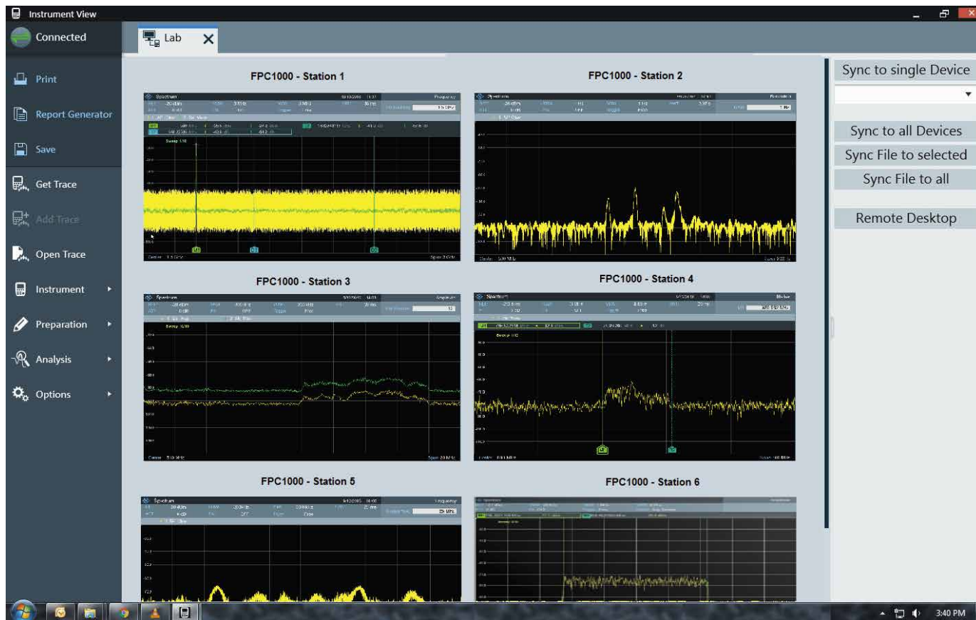
Fig. 2: The LabView function in the R&S®InstrumentView remote control software is used to manage multiple R&S®FPC1000 spectrum analyzers in a Wi-Fi network.
